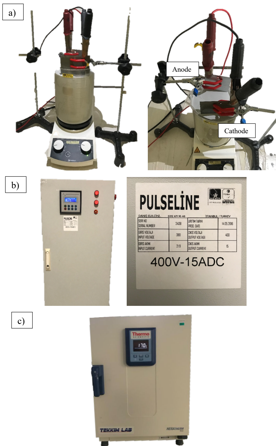
Figure 3.1 Test Setup; a) Reaction Bath; Anode and Cathode b) Rectifier 0-400V c) Oven 250 °C
